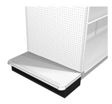
End Deck locks onto Base End Trim and can easily be removed by releasing locking clips. No tools are required and the End Merchandising Panel does not need to be removed to install or release End Deck.
