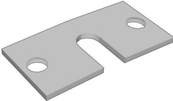
Base Bracket Anchor Plates are required when your fixture exceeds height-to-depth ratio limits and for fixtures over 5' tall in certain seismic zones. The plates secure each Leveling Leg to the floor using anchor bolts.
