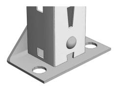
Use Uprite Frame Anchor to secure Uprite Frame to floor. Anchor is required when height-to-depth ratio exceeds 6 to 1 and to meet certain seismic anchoring specifications. Includes Uprite mounting hardware, but Anchor bolt is not included.
